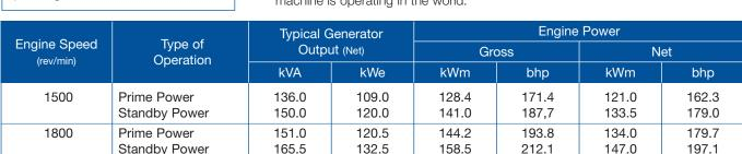
All ratings data based on operating under ISO/TR 14396/ISO 8528 conditions using typical fan sizes and drive ratios. For operation outside of these conditions please consult your Perkins contact. Performance tolerance quoted by Perkins is +5%. Electrical ratings assume a power factor of 0.8 and a generator efficiency of 90%. Fuel specification: BS 2869 Part 2 1998 Class A2 or ASTM D975 D2 Lubrication oil: A single or multigrade oil to ACEAE1 E2 or API CD/SD
